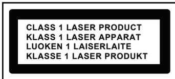
Class 1 laser product label - This label is attached to the place as illustrated to inform that the apparatus contains a laser component.
