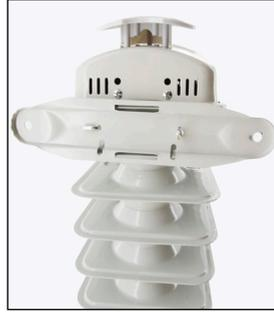
5. Screw the wing nuts back to the U-shaped bolt and fasten the wing nut properly.
