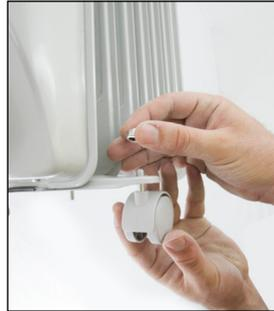
6. Screw off spherical nut from the castor, align the shaft to the hole of the castor mounting plate, insert in and screw on the spherical nut.
